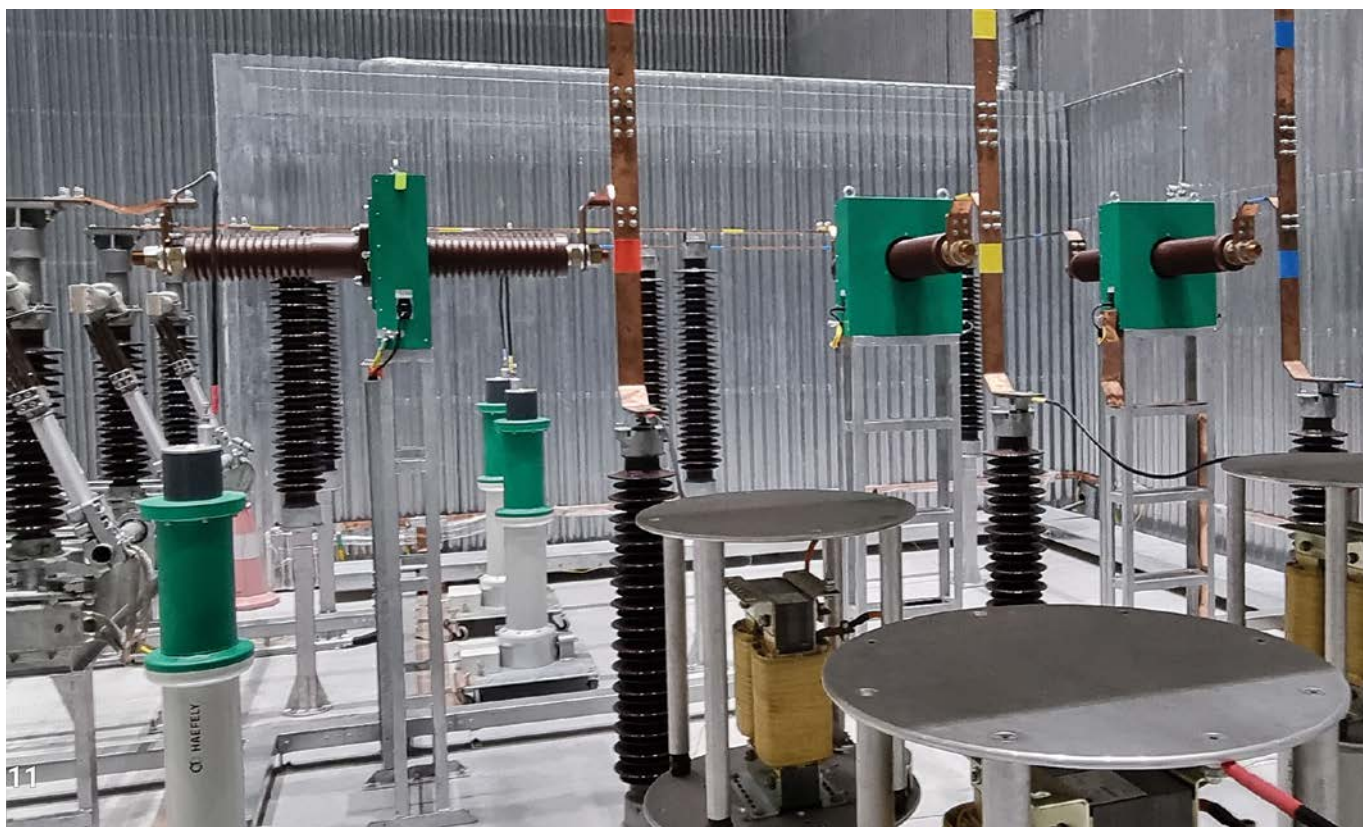
TMS 580 100 kV 3000 A: Transformer Loss Measuring System
