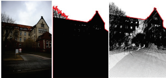
Figure 5 Skyline feature extraction from images and laser scan data. Left photograph is the original image, middle photograph represents threshold image (black pixels represent objects and white the sky) and the right photograph is the laser scan coloured by intensity.
