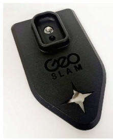
Figure 9 Reference plate for handheld mobile mapping systems. The system is placed on a reference point in a way that the cross coincides with the point marker. The positional offset between the centre of the cross and b-system of mobile mapping system needs to be known.
