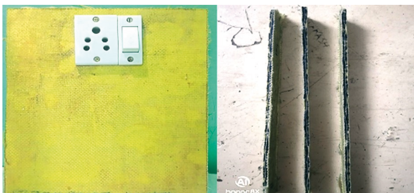
Fig. 6 Electrical board and automotive door panel application of composites
