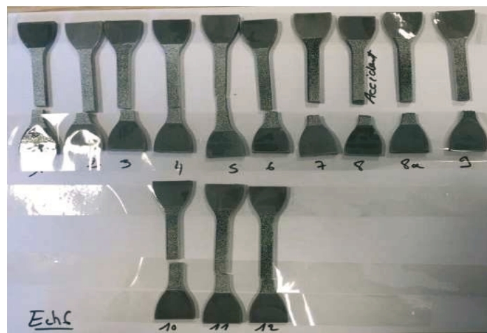
Fig. 2 Typical failure mode of PVC specimens
