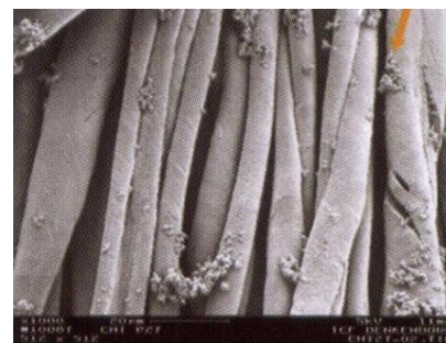
Fig.5 SEM image of alkaline earth fine crystalline sediment from a bath that does not contain carbonates, magnification 1000x [59]
