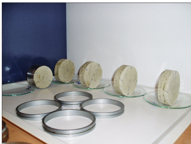
Figure 1: Undisturbed samples of swelling material from the Muvrinski Jarak location
