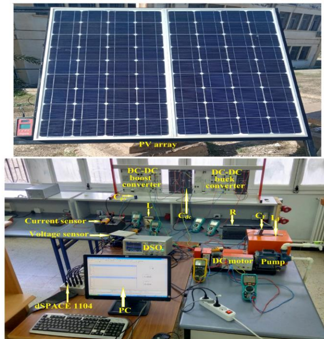
Figure 7. Experimental test bench based on dSPACE 1104.
