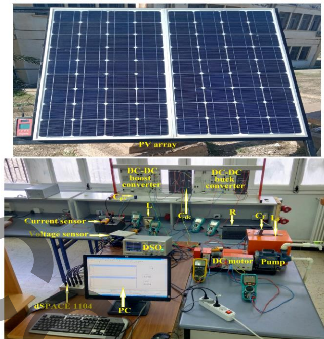
Figure 7. Experimental test bench based on dSPACE 1104.
