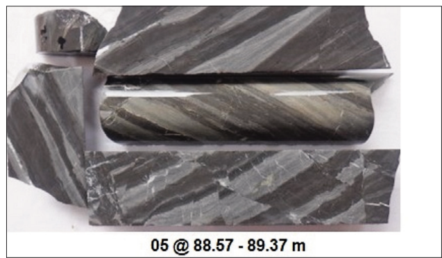
Figure 5: Cut drill core sample photo of silty tuff with sandy tuff intercalations
