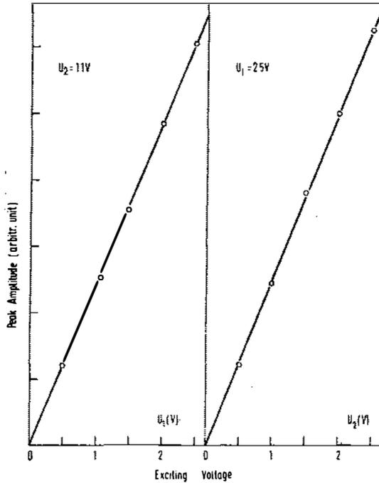
Fig. 3. The peak amplitude of the  $f_1 - f_2$  wave as a function of the exciting voltages of the  $f_1$  and  $f_2$  waves.
