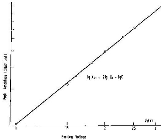
Fig. 5. The peak amplitude of the  $2f_1$  wave as a function of the exciting voltage of the  $f_1$  wave.
