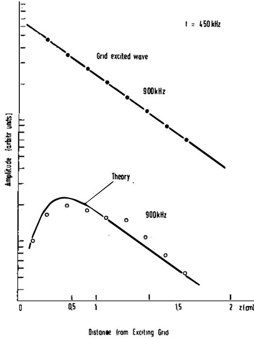
Fig. 4. The amplitude of the  $2f_1(0)$  wave as a function of distance from the exciting grid. The amplitude of the grid excited wave (●) is also shown.
