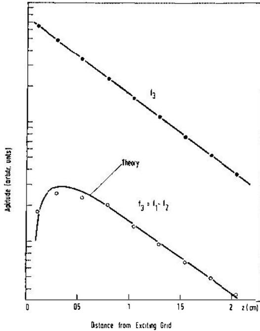
Fig. 2. The amplitude of the  $f_1 - f_2(0)$  wave as a function of distance from the exciting grid. The amplitude of the launched  $f_3 = f_1 \cdot f_2$  wave is also shown.
