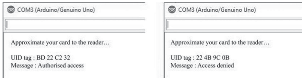
Figure 8. RFID tag access checking with the reader module.
