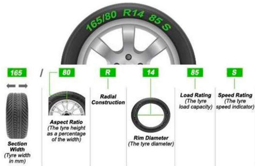
Figure 1. Overview of pneumatic tire specification.
