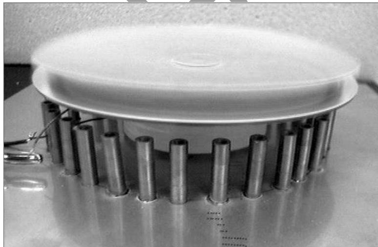
Figure 9(a). Depiction of the mirror's concavity during its rotational phase, influenced by the activation of the electromagnets, evidenced by the protrusions beneath the revolving mirror surface.
