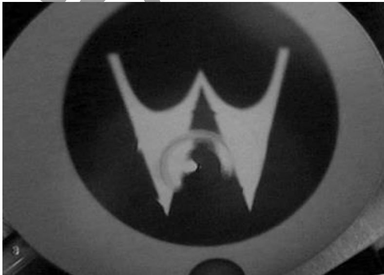
Figure 14. Sharpened image achieved by the mirror upon supplying the appropriate voltage to the electromagnetic components.
