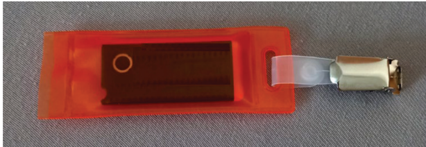
Figure 1. A thermoluminescent personal dosimeter
