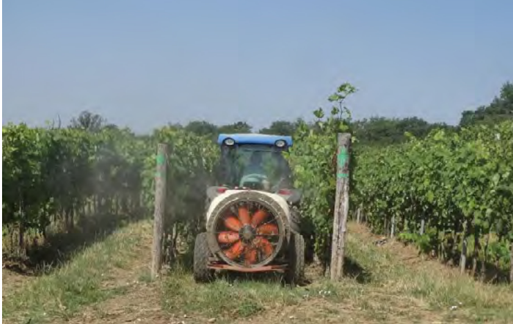
Slika 3: Aksijalni orošivač Friuli Sprayers ATV 1000 Figure 3: Friuli Sprayers ATV 1000 axial air-assisted sprayer
