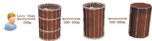
Figure 6 Schematic diagram of distance control LOD layered loading
