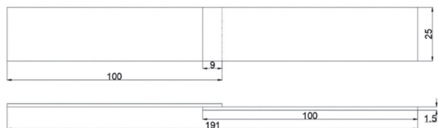
Figure 1 Schematic presentation of a test sample
