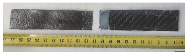
Figure 2 Test sample after being tested in a tensile testing machine
