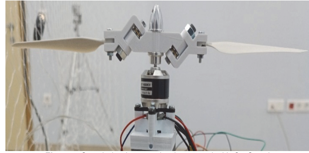
Figure 5 Swashplateless mechanism tested with Co-Stand
