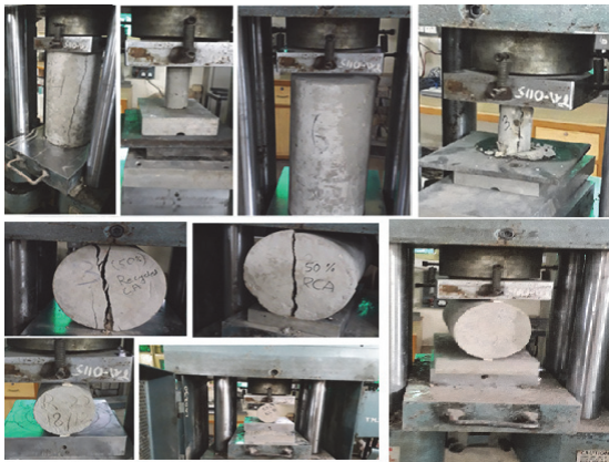
Figure 4 Selected specimen for compressive strength and split tensile strength testing
