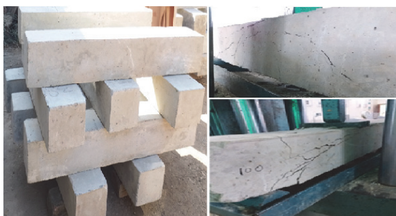
Figure 5 Selected RC beams for flexural strength testing
