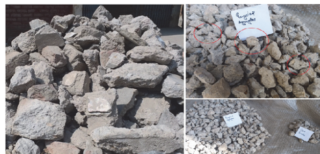
Figure 2 Concrete Blocks of C&D waste and cracked particles of RCA
