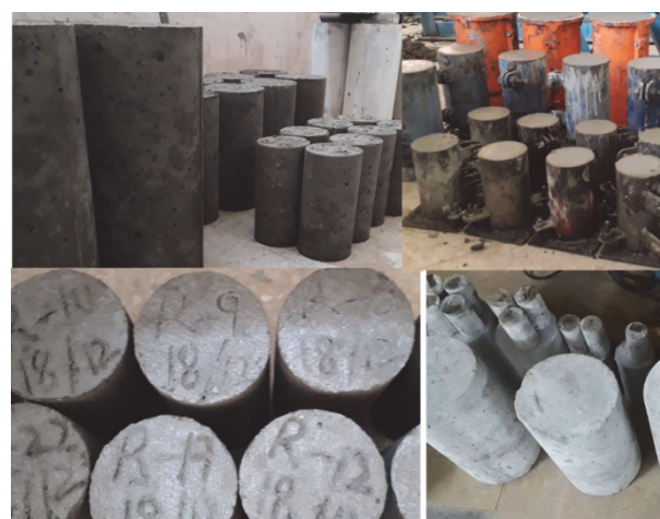
Figure 3 Different size of cylinders before testing
