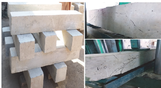
Figure 5 Selected RC beams for flexural strength testing
