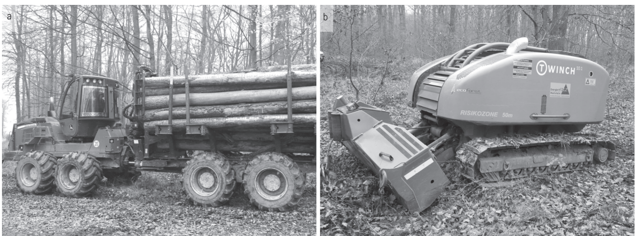
Fig. 1 8-wheel forwarder John Deere 1510G (a) and traction aid winch Ecoforst T-Winch 10.1 (b) used in the trial. The image of the forwarder shows the softwood logs carried during the experiment. The winch is pictured in working position, with the blade lowered against a stump for securing the machine in place during traction assistance
