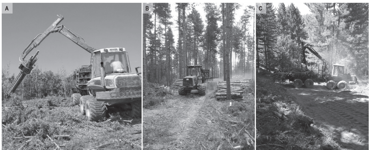
Fig. 5 Forwarders tested (A) Ponsse Gazelle, (B) John Deere 1420, and (C) John Deere 1110D working in site A, B, and C, respectively
