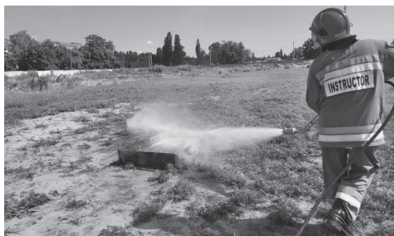
Figure 14. Extinguishing a simulated fire of a "B" class at the final stage during the III series of studies
