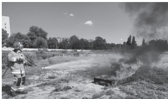
Figure 13. Extinguishing a simulated fire of a "B" class at the initial stage during the III series of studies
