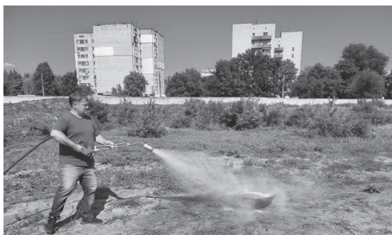
Figure 12. Extinguishing a simulated fire of a "B" class at the final stage during the II series of studies
