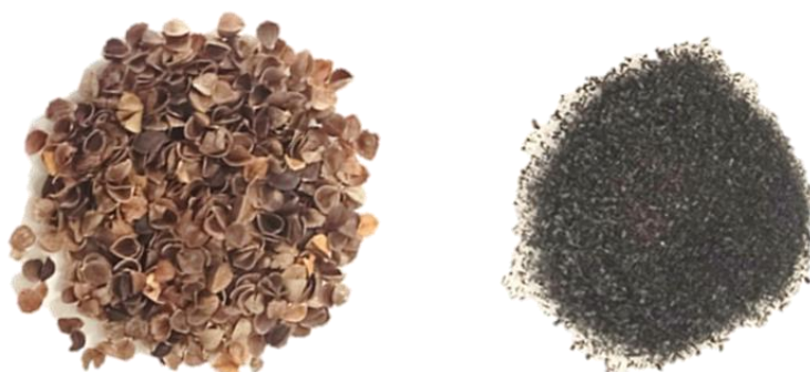
Figure 1. Physical appearance of unmodified buckwheat hulls alongside biochar derived from buckwheat hulls
