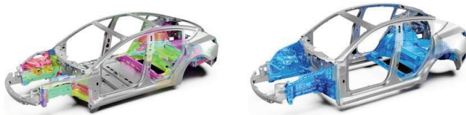
Figure 2 Change of car body parts due to large die casting a Tesla Model Y [6]
