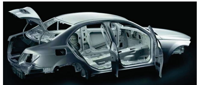
Figure 1 Body with self-supporting shell construction ([3], p.18)
