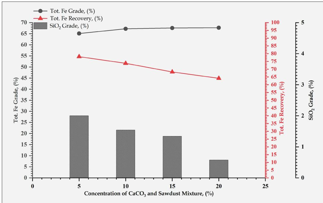
**Figure 8:** Effect of CaCO<sub>3</sub> and sawdust mixture concentration on tot. iron grade, tot. iron recovery and silica content
