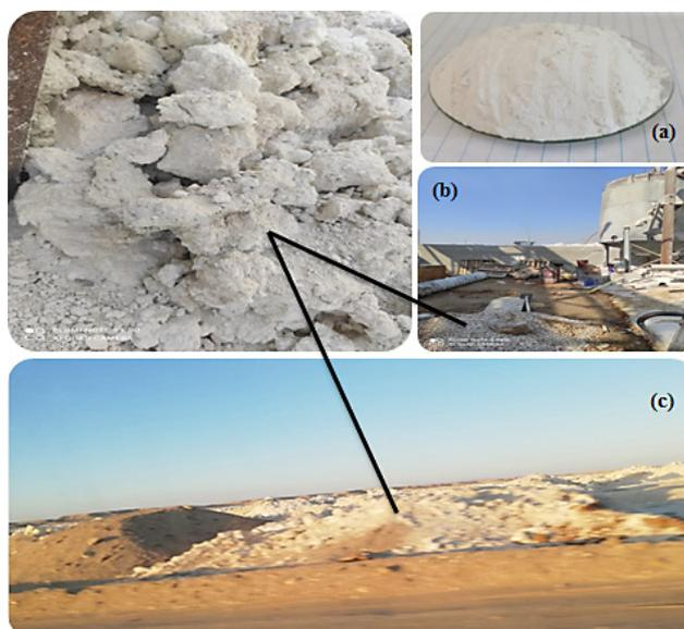
**Figure 2:** a) Paper industry sludge (calcium carbonate waste) after being ground in a mortar, b) Calcium carbonate waste within the Quena Paper Industry Company, c) Quena Paper Industry Company sludge dump abroad.
