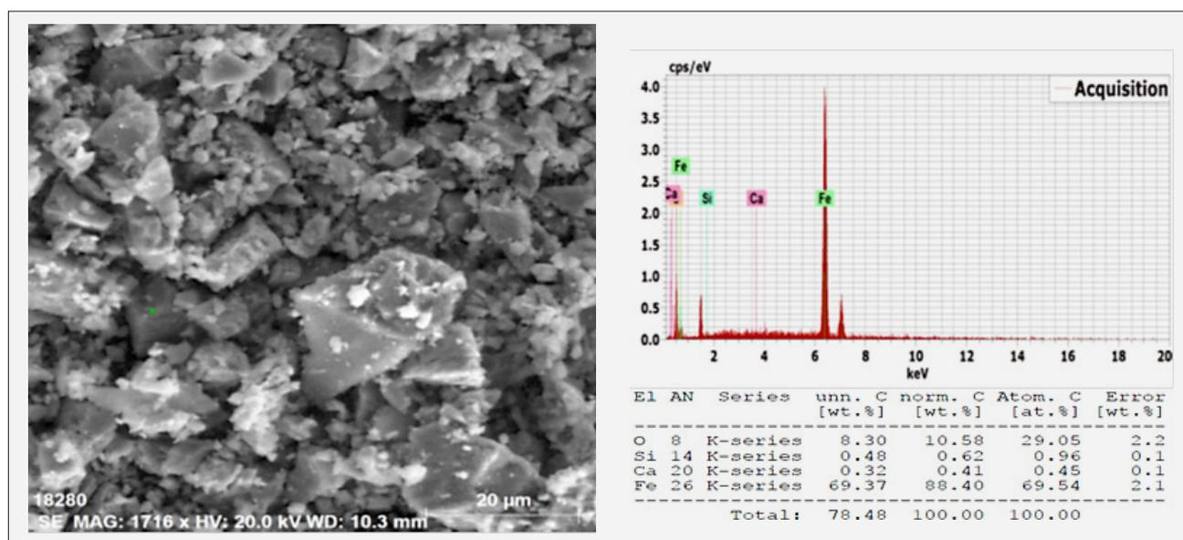
**Figure 13:** SEM-EDS results of reduced and separated Um Nar BIF with a 10% dosage of mixture of CaCO<sub>3</sub> and sawdust
