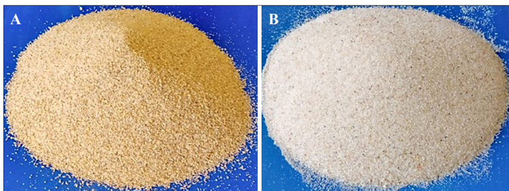
Figure 8: Classified head sample before (A) and after (B) attrition
