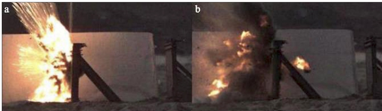
Figure 7: EFP projectile hitting target (Kurzawa et al., 2018)
