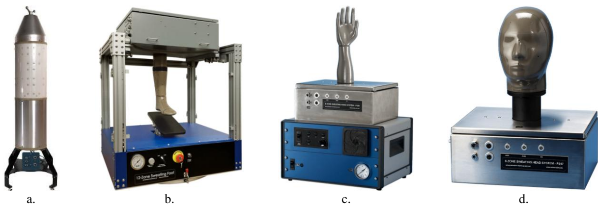
Fig.9 Anatomically shaped measuring instruments for measuring thermal insulation: a. thermal torso; b. thermal foot; c. thermal hand and d. thermal head [58]
