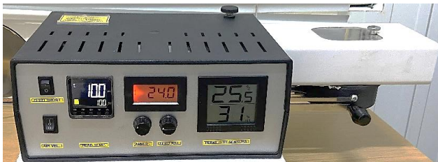
Fig.8 Measuring instrument for non-destructive measurement vapour permeability and water vapour resistance - Permetest
