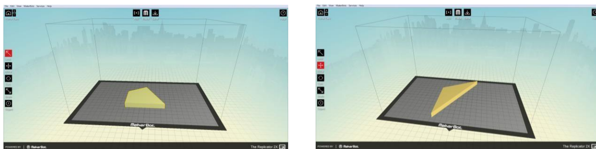
Fig.3 Positioning of test objects on the printer base
