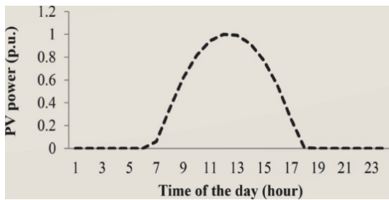
Figure 4 An average everyday solar electricity production curve adjusted to the morning's peak production
