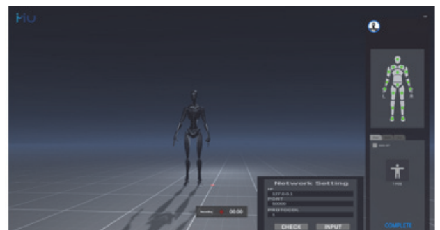
Figure 5 Appearance of a 3D avatar in the Unity engine program mapped based on sensor data of 15 major joint points
