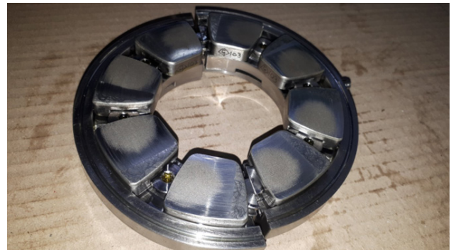
Slika 3. Matirani sloj na segmentima odzivnog ležaja Figure 3. Matted layer on the thrust bearing segments
