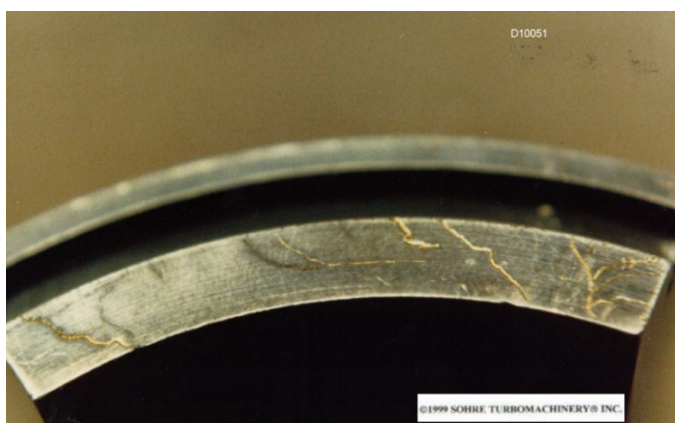
Slika 6. Tragovi iskrenja na segmentu nosivog ležaja [4] Figure 6. Traces of sparking on the bearing bearing segment [4]
