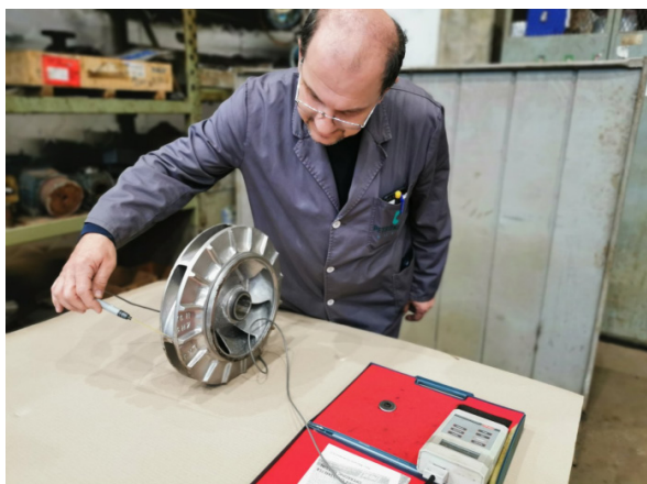
Slika 10. Mjerenje zaostalog magnetizma Figure 10. Measurement of residual magnetism
