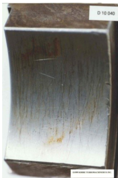
Slika 5. Tragovi iskrenja na segmentu nosivog ležaja [4] Figure 5. Traces of sparking on the bearing bearing segment [4]
