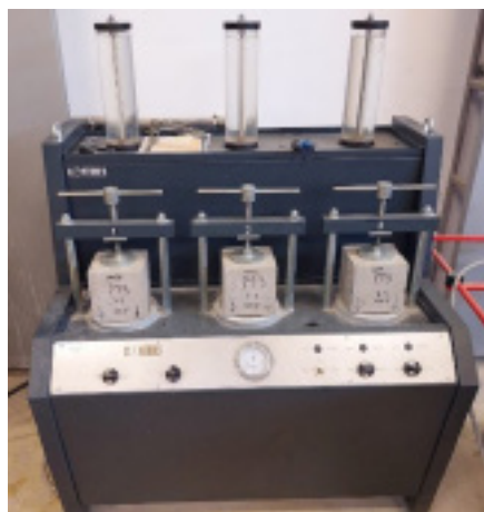
Slika 6. Ispitivanje dubine prodora vode pod tlakom Figure 6 Test of water penetration depth under pressure
