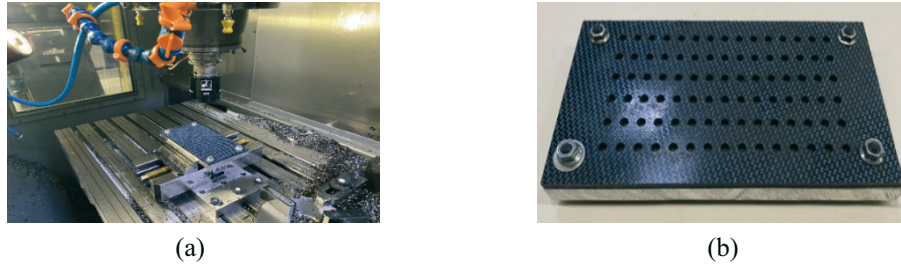
Fig. 12 (a) Pre-stack drilling view of the composite and AA7075 fixed on the CNC Vertical Machining Centre; (b) Post-stack drilling view of composite and AA7075
