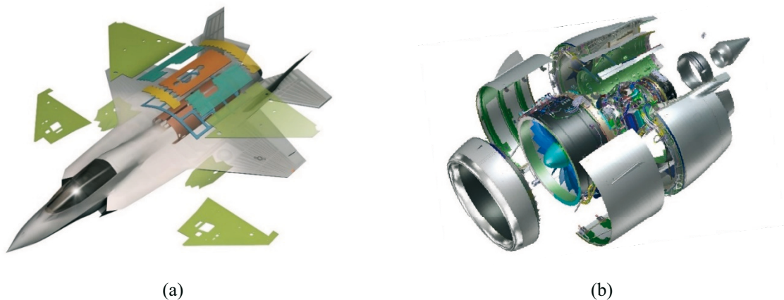
Fig. 2 (a) Some composite parts used in the F-35A fighter fuselage [7]; (b) Some composite parts used in the aircraft engine [8]
