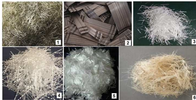
Figure 1 Different fibers types: 1,2-Steel; 3-Glass; 4,5-Polypropylene-PP; 6-Banana fiber
