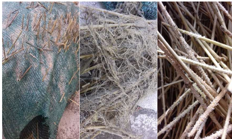
Figure 3 The bag with branches, dry branches, and the remaining woody part of the branches (sample B)
