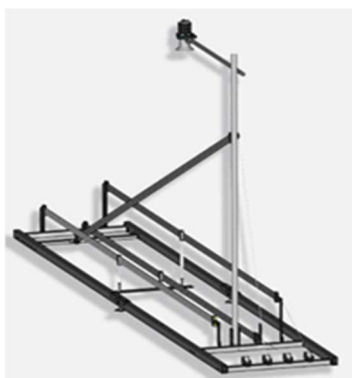
Figure 9 Snow density measurement device, SOMMER SPA-2 (AAXIS NANO TECHNOLOGIES PVT. LTD. 2024)
