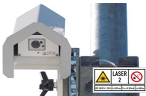
Figure 5 Snow height measurement device, Lufft SHM31 (Lufft an OTT HydroMet brand 2024)
