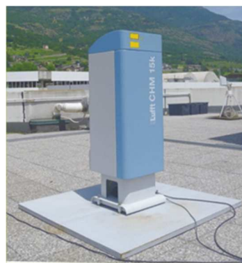
Figure 10 Cloud base height measurement device, Lufft CHM 15k Ceilometer (ResearchGate 2024)
