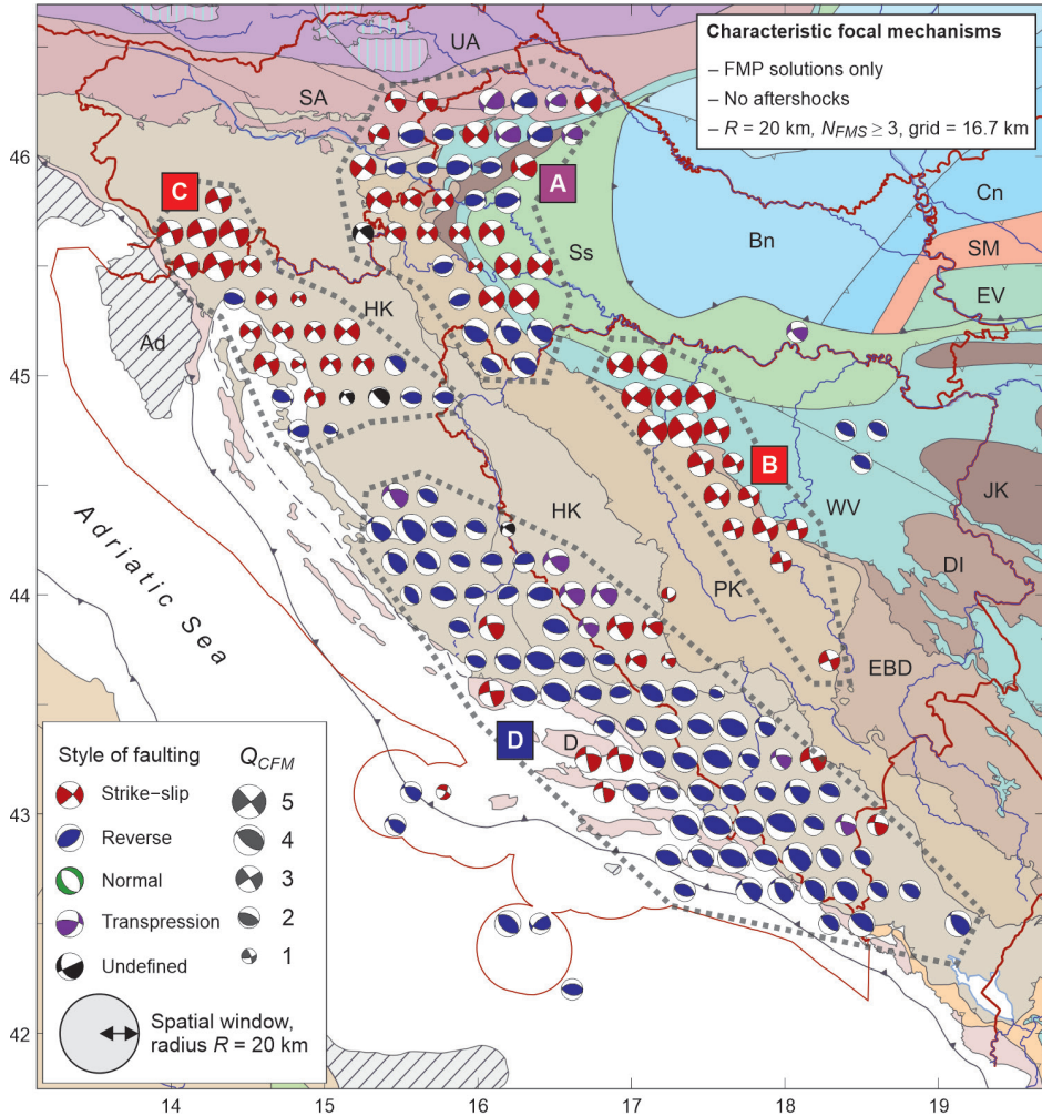
Figure 15. Characteristic focal mechanisms (CFM) computed by weighted averaging of the FMP focal mechanisms on a grid 16.7 \text{ km} \times 16.7 \text{ km} , within the spatial window with radius of R = 20 \text{ km} . Aftershocks were not considered. Only solutions based on at least three events in the window are shown. The size of the beachballs scales with the quality Q_{CFM} . The basemap of tectonic units is simplified after Schmid et al. (2020, see caption of Fig. 7 for detailed explanation).
