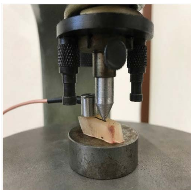
Figure 5. AE sensing during metal indenter penetration
