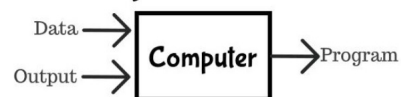
Figure 2: Conventional Programming vs Machine Learning: Machine learning as automating the process of automation, in contrast to traditional programming, which merely reflects automation.
