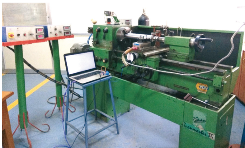
Fig. 5 Experimental turning centre – a Kirloskar Turnmaster 35 lathe
