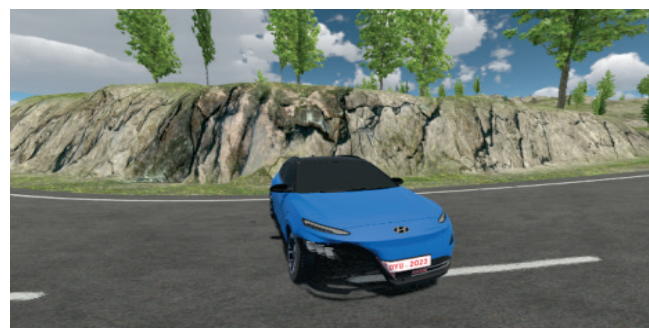
Figure 10 Implementing car body damage from collisions. Adjusting the parameter values in the Damage options can change the amount of damage.
