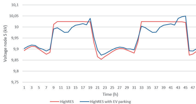
Figure 26. Voltage at node 5 during February for HighRES scenario
