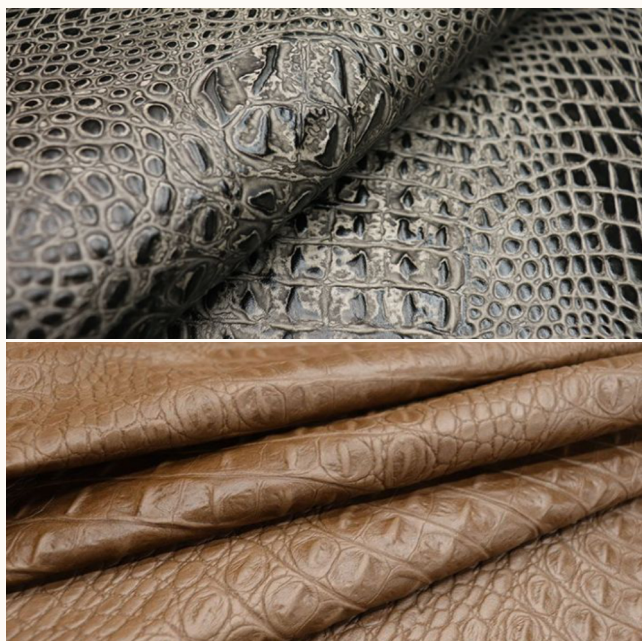
Figure 1. Embossing the leather face: a) on a press, b) on roller [10]
