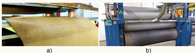
Figure 1. Embossing the leather face: a) on a press, b) on roller [10]
