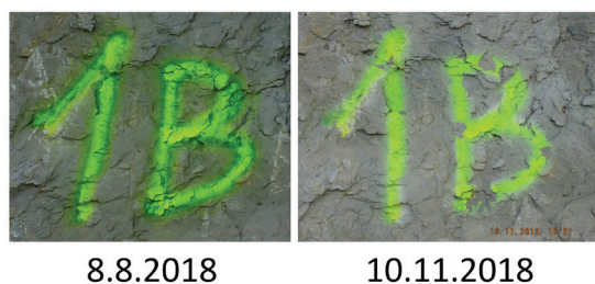
Fig. 9. Lettering on the polygon 1B is severely degraded in 94 days of exposure, and had to be repainted during each measurement campaign.
