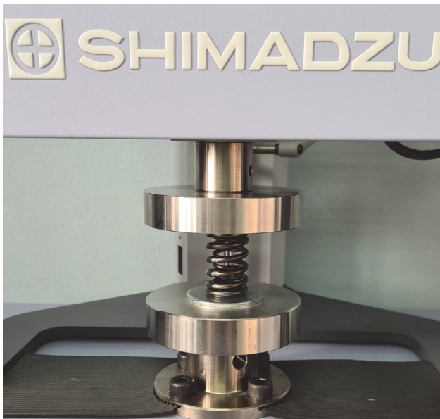
Figure 4 Measurement of valve compression force
