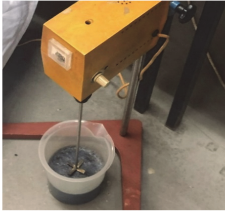
Figure 2 Preparation of nano-fluid for cooling and lubrication
