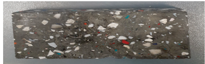
Figure 14 Test sample created in the composition 85 concrete/15 plastic
