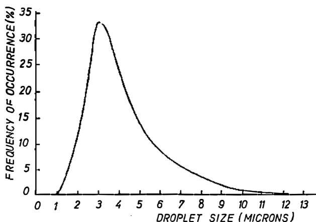
Fig. 2. Cloud droplet size (radius) distribution determined from soot coated slides.
