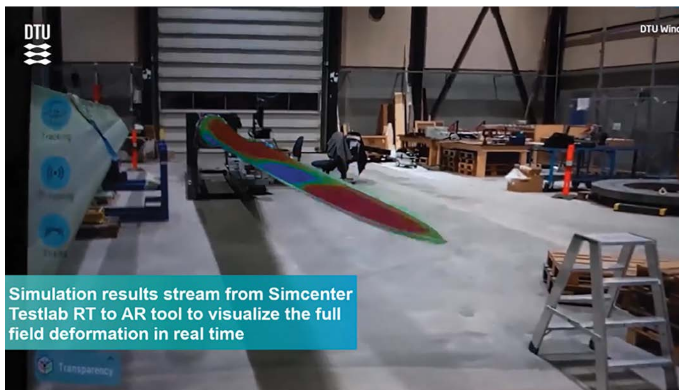
Figure 6. Simcenter real-time AR visualization of the deformation of a wind turbine blade
